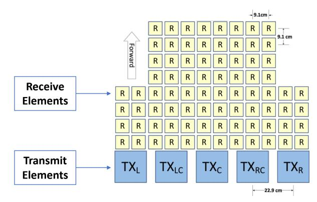
Two-dimensional synthetic aperture allows formation of three-dimensional sonar imagery
