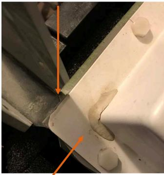
Crack on clamshell caused handle pressure (repaired in-field with JB Weld)
