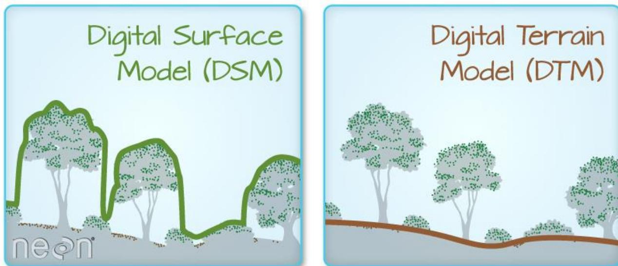
**Figure 9 Distinction between a DTM and DSM**
