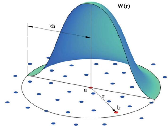
Particle approximation in SPH method
