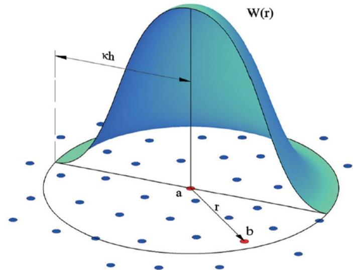
Particle approximation in SPH method
