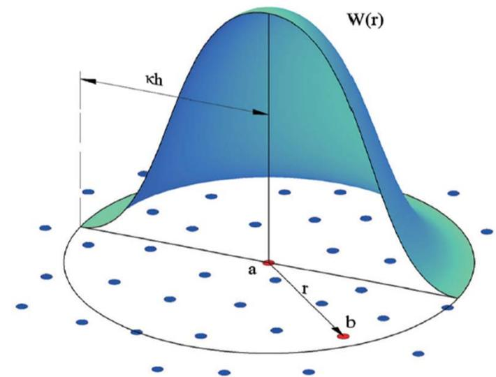
Particle approximation in SPH method
