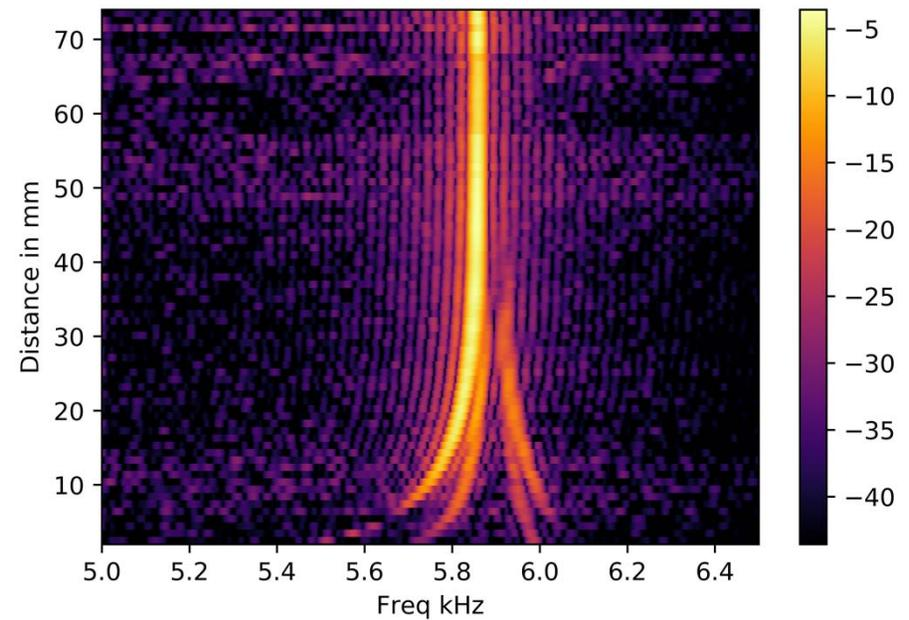
First bending mode is at 5900 Hz
