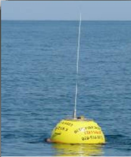
FRF 17m Datawell Waverider Buoy
