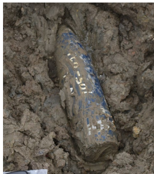
Inert 105mm Projectile Depth: 1.3m Burial: 6cm
