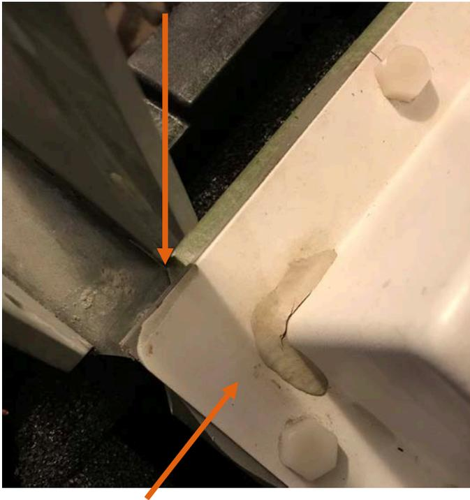
Crack on clamshell caused handle pressure
