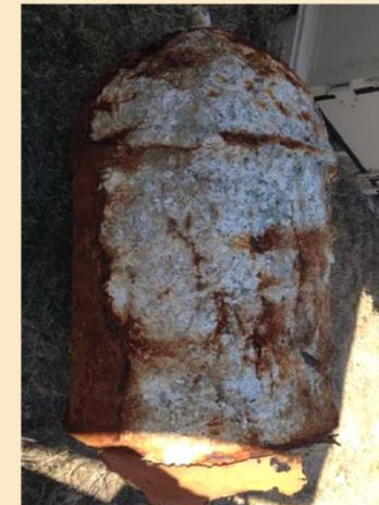
EOD visual inspection revealed 6ft cylindrical object with cable on one end, open on other end, and with sand inside. Assessed not to be an immediate hazard.
