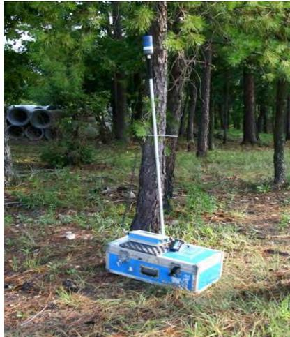
Figure 6-2: Geometrics G-856 Proton Precession Magnetometer
