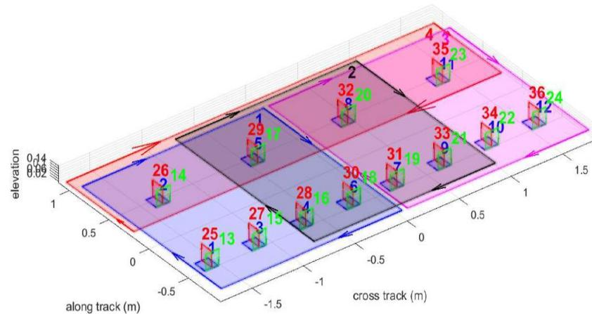
The UltraTEMA system consists of four transmitter coils and twelve vector receiver sensors. It measures complete EMI response of a target at each dynamic data point and provides 144 data value at each  $n^{\text{th}}$  ( $n=1,2, \dots, 25$ ) time gate.
