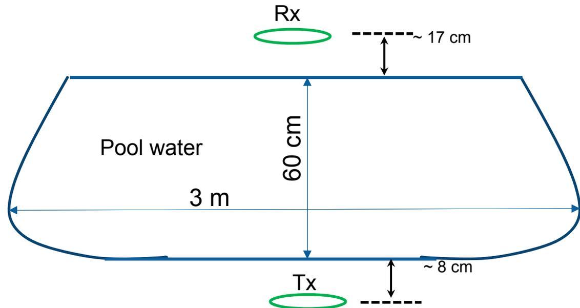
HFEMI Tx & Rx coils are about 27 cm in diameter, 12 turns. Approx distances from the coil centers to the upper and lower water surfaces are indicated.
