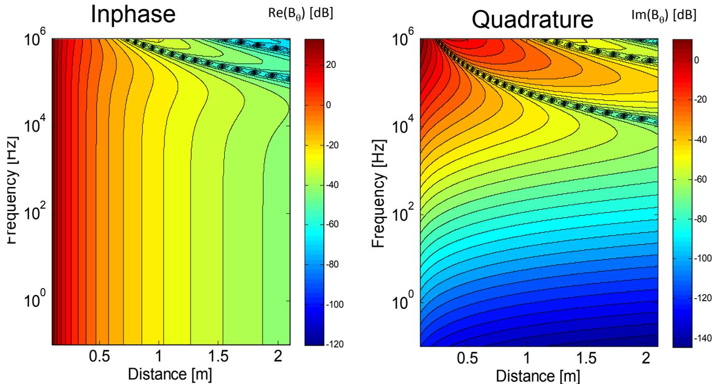
A magnetic  $m_z$  dipole placed in ( $\sigma = 4$  S/m) as a function of frequency (y-axis) and distance (x-axis).
