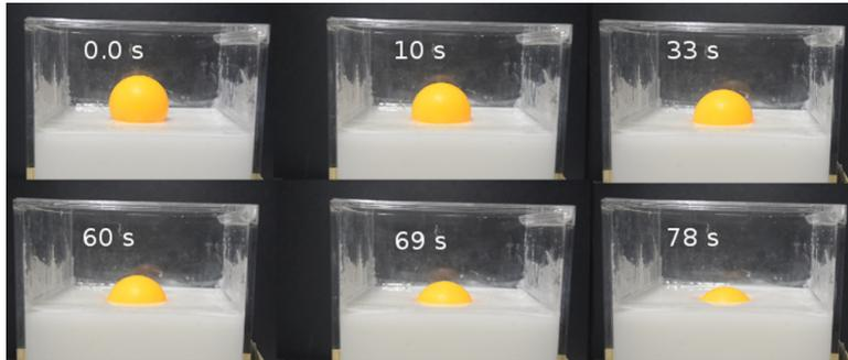
$$\Delta B(t) = (D_{\text{obj}}/\text{frict}_{\text{coeff}}) (\rho_{\text{obj}}/\rho_{\text{sed,wet}} - 1) \Delta t$$
