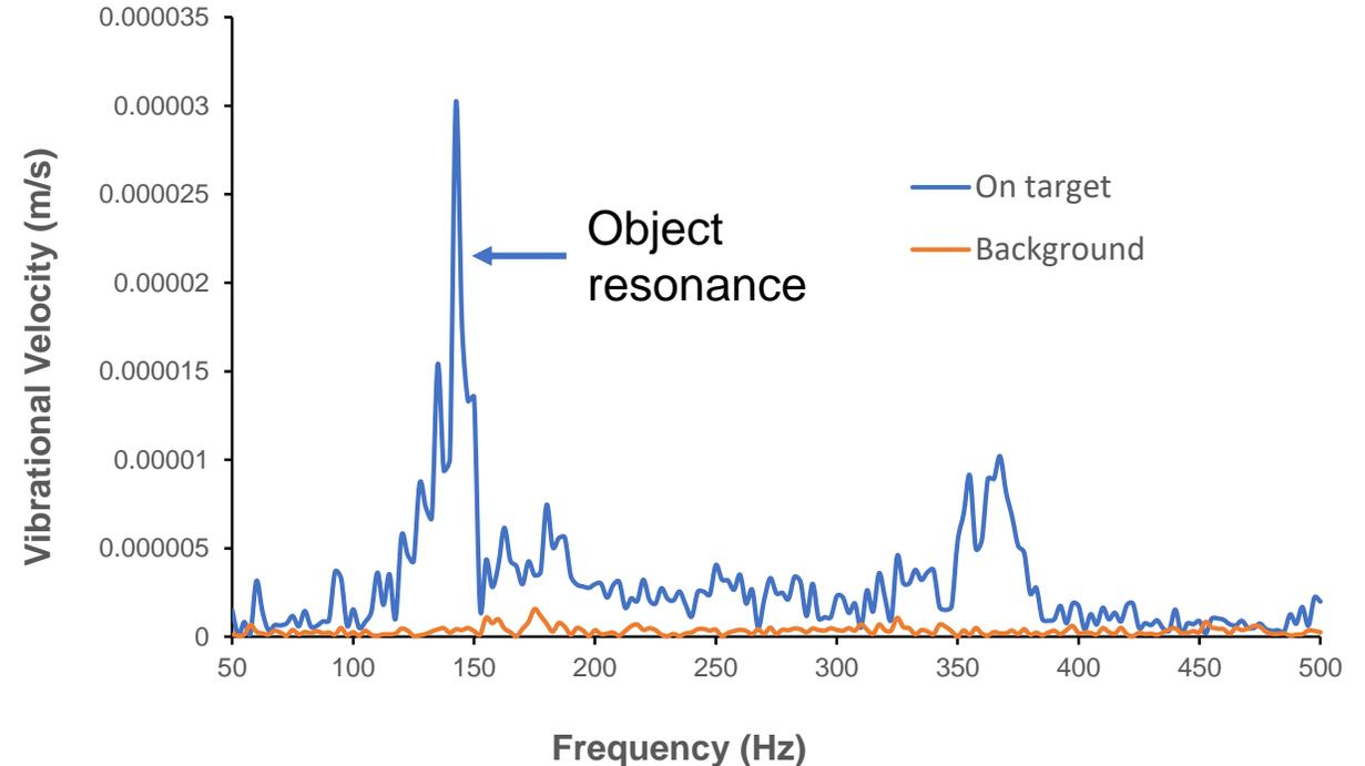
Spectrogram of vibrational velocity for points on and off target
