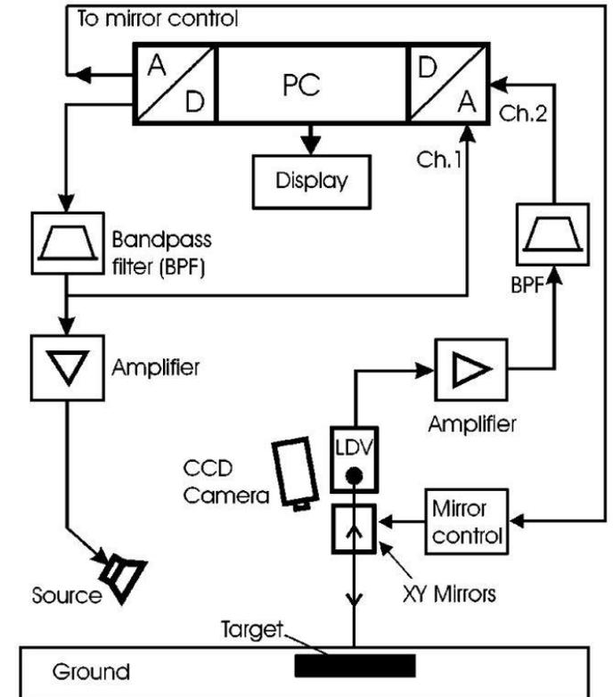
Schematic diagram of the measurement system using LDV (Sabatier, 2001)
